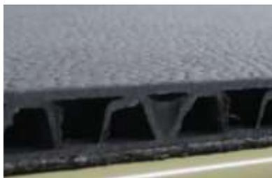
The load compartment floor consists of a three-dimensional center layer with bubble structure on which a TPO film (thermoplastic polyolefin) is laminated. The TPO film is durable, stain-resistant, slip-resistant and has low wear. The bubble structure of the center layer ensures a low weight while offering strong rigidity and good damping properties. Below that is an insulating foam layer. Support bars connect it to the vehicle floor. The plastic floor has a thickness of
