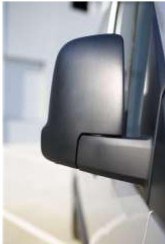
With code FU5, the exterior mirrors are fitted without turn signal indicators. Due to the omission of the indicators the mirror housing is not as wide, thereby overall width of the vehicle is reduced by approx. 0.78" (20 mm) each side. Other dimensions and the geometry of the mirror glass, also in combination with code FS2, extra-long mirror bracket, remain identical with those of the serial exterior mirrors. The mirror heating, code F68 as well as F64, is not available.
