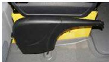
Installation of an adjustable parking brake lever. This parking brake lever can be lowered even when the parking brake is on.
