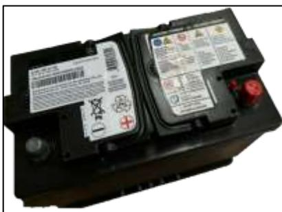
A heavy-duty 12 V/92 Ah AGM (Absorbent Glass Mat) starter battery is fitted instead of the standard starter battery. The AGM battery is smaller and lighter than common batteries, because the energy density is increased.
