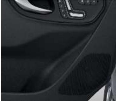
2 tweeters are fitted on the outside. Depending on the configuration, an additional speaker is fitted in the centre of the instrument panel, 4 more speakers are located in the side trim of the passenger or cargo compartment. 6 bass/mid-range speakers are fitted in the driver's and co-driver's door as well as in the left and right side trim in the rear.
