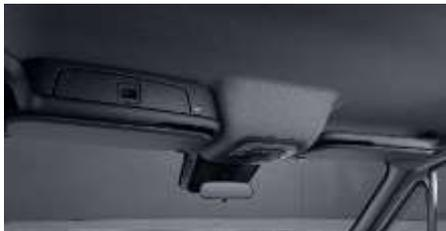
The lockable compartment, code FQ6, is placed on the driver's side above the windshield and complements a shelf. The hatch (approx. 13" x 3" (330 x 77 mm) opens upwards and remains in position. It can be locked using the emergency key attached to the key fob. The maximum dimensions of the lockable unit correspond to the size of the shelf is approx. 22.83" x 10.63" (580 x 270 mm).
