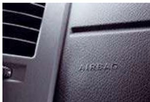
The passenger airbag unit is located in the right side of the instrument. The passenger airbag is available for an individual seat, for a bench seat (S23) and only as a twin passenger airbag version. In an accident it is inflated within milliseconds by a gas generator, reducing the risk of the seat occupant's head or chest impacting the steering wheel during a frontal collision.
