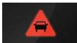
The Active Brake Assist with cross traffic function continuously checks for a safe distance of the vehicle in front and warns the driver both optically and acoustically of potential collisions (e.g. rear-end collision) with other vehicles, significantly reducing the risk of accident.
