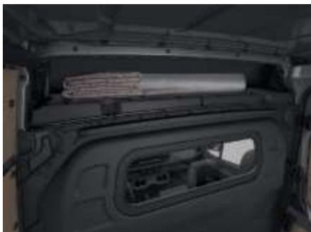
The storage compartment above the roof paneling uses the space between the headliner of the cab and the vehicle's high roof (D03) as an additional storage facility. The compartment is accessible from the loading area and can support a load up to 77 lbs. (35 kg).
