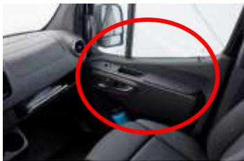
The cushioned armrests on the driver's and co-driver's door, code S28, are optionally available. The faux-leather armrests offer an increased level of comfort and are mounted behind the door switch and handle.
