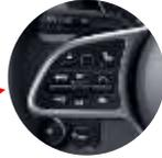
The cruise control accelerates and brakes the vehicle automatically in order to maintain a previously stored speed above 15 mph (24 km/h). The cruise control is operated using the left steering wheel buttons. A limiter function is not available. If the cruise control is activated and the optional available Traffic Sign Assist has detected a speed restriction sign, the maximum permissible speed displayed in the instrument display can be stored
