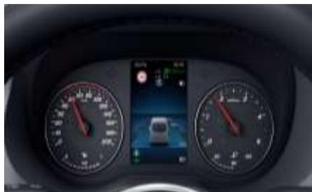
DISTRONIC regulates the speed and the distance of the vehicle with a short and long range sensor located in the front bumper. The system regulates automatically according to the specification set by driver; it brakes when necessary and accelerates again when possible. In slow moving or stop/go traffic, the DISTRONIC brakes the vehicle automatically (if necessary to a standstill). Once the traffic situation allows moving again, the DISTRONIC accelerates the vehicle automatically up to the set
