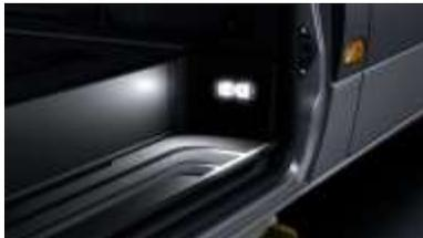
The exit lights are integrated in the driver's and passenger's door and in each step trim of the sliding door. The exit lights of the step trim come as LED variants and the lights of the doors come as conventional bulbs. As the doors swing open, the exit lights illuminate the ground for safe boarding and alighting.
