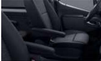
A tilt-adjustable armrest is fitted to the inboard side of the co-driver's backrest. Retrofitting this armrest entails swapping the entire backrest.
