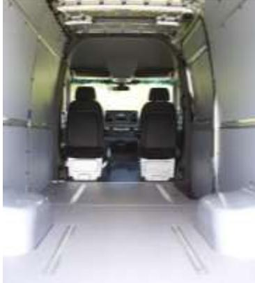
No partition is installed on cargo vans. B-pillar is wrapped but the retrofit of a bulkhead is still possible.
