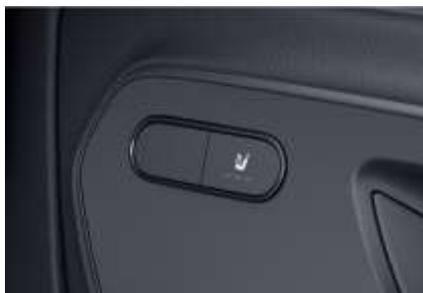
The heated seats are equipped with heating filaments in the seat cushion and backrest which are controlled by three-stage switches in the front door panels. When stage three is turned on for rapid heating, the system will run for approx. 7 minutes then automatically switches to stage two. After approx. 10 minutes, the seat heating automatically switches to stage one. The seat heating is automatically switched off after a further 20 minutes. It can be switched off manually at any time.
