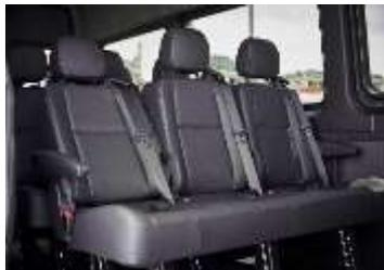
A three-seater comfort bench is fitted in the **second** row of the passenger compartment. All three seats are fitted with a three-point seat belt and have additional seat bolster padding, allowing for enhanced seating comfort. Each row is individually reclinable as well as an individual recliner setting on each seat.
