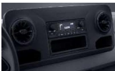
The 1-DIN radio with FM/AM reception comes with an LCD display and an integrated USB-C port. The radio can be operated exclusively via the device itself and not via the optional multifunctional steering wheel.
