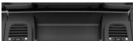
Two additional air vents are installed in the center storage compartment on the instrument panel. These vents are adjustable and distribute exclusively cooled air. Heating up is not possible in this case.
