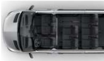
A three-seater bench is fitted in the **second** row of the passenger compartment. All three seats are fitted with three-point inertia-reel seat belts. ISOFIX child seat attachment points are on the two outer seats.
