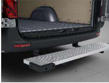
The code W75 includes a hot-dip-galvanized steel step fitted at the rear of the vehicle. The step measures 63 x 11,81" (1,600 x 300 mm) (width x depth). Solid rubber mouldings on the outer corners provide protection when manoeuvring.
