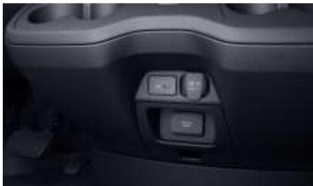
The 5-Volt USB-C power socket is located centrally in the lower part of the cockpit, below the center cup holder and next to the standard 12-Volt socket. Allows for these options to be within easy reach of driver and passenger.
