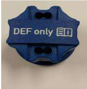
This code includes a blue filler cap for the DEF tank and a plastic key element for diesel engines. To lock or unlock the filler cap the dust protection must be turned to the side and the key element needs to be inserted. This makes it possible to turn and remove the DEF filler cap. After the DEF tank has been filled and closed, the key element can be removed. The key element is with the tool kit enclosed in the storage compartment on the passenger's foot well.
