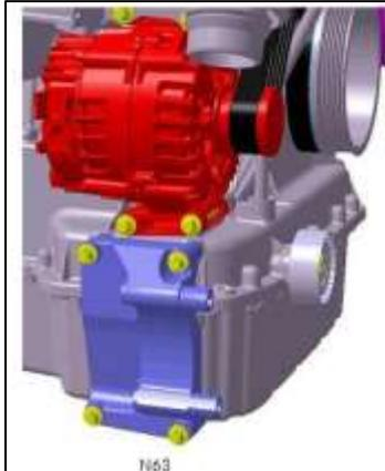
It is possible to attach an additional auxiliary alternator on the right side of the engine next to the oil pan, but this must be done using the factory option N63 as the bracket.
