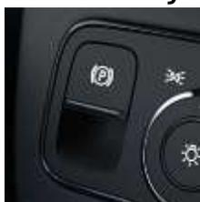
The release automatic parking brake function is performed as soon as a sufficient level of driving torque is applied to the wheels on the front or rear axles to enable the vehicle to drive off. If the electric parking brake switch is operated and held when driving, the ESP unit recognizes a braking request which results in braking via a service brake. The instrument cluster displays a message and a warning tone is sounded.
