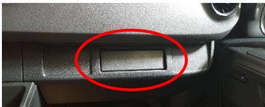
When ordering code FE9 a 1-DIN slot is included underneath the dashboard on the co-driver’s side. This slot can be used for additional electronic devices. It comes with a cover for delivery and includes a cable set which reaches into the slot and offers the following connections:
