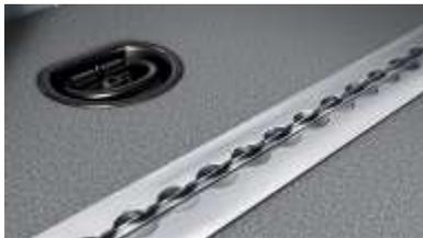
The load securing rail system includes two rails that are attached to the floor in the load compartment. Each load securing rail is configured for a maximum tensile loading of 1124 lb.ft/500 daN. Straps are not included in the specification, but are available as accessory.
