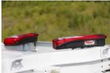
The wiring harness of both tail lights are approx. 78.7” (200 cm) longer than the standard one. They are rolled up and provisionally fastened at the rear frame end and allows upfitters to fit taillights easier in a different position.
