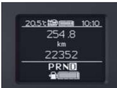
The temperature sensor is mounted in the front bumper and displays the current outside temperature in the instrument cluster.
