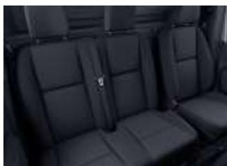
With code S23, a twin seat is installed on the passenger’s side instead of a single seat, allowing an additional seat for a third person. Both seats are equipped with three-point seat belts and head restraints. The seat cushion can be completely folded forward and therefore it’s possible to use the seat frame as a storage compartment.
