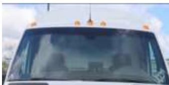
Vehicle marker and clearance lamps are required by law on all vehicles with a total width of 80" (203 cm) and above according to FMVSS standards. The five identification lamps are mounted in the area of the windshield at the vehicle roof. The two outer ones are used as clearance lamps and the three inner ones are identification lamps. The preparation
