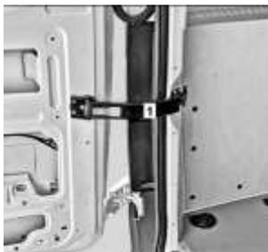
When loading and unloading on an incline or, for example, in strong winds: additional blocks allow the rear doors of the Sprinter to be mechanically fixed at an angle of 90°. This facilitates access to the load compartment and ensures that the rear doors do not close unintentionally.
