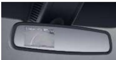
For passenger, cargo and crew vans with the standard radio E10, the rear view camera FR3 is standard. This camera will display the area behind the vehicle, with the image appearing in the rear view mirror. This allows the vehicle to display areas that are not commonly visible to the driver. The image appears in the rear view mirror when shifting to reverse gear. The reversing camera switches off automatically when the vehicle is driven in forward direction.
