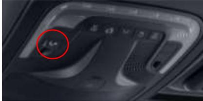
By pressing the breakdown assistance button, a voice connection to the service center is established in order to be able to initiate assistance quickly and effectively in the event of a defect with the vehicle.
