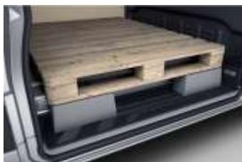
A pallet support is available for the standard step in the load compartment (sliding door). The two plastic inserts are latched onto the step and close the gap between the closed sliding door and the floor of the load compartment.
