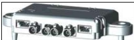
Upfitters can install their own antenna and use the antenna interface to connect the telematics. This enables exchange of analogue and digital radio signals as well as GNSS and GSM signals and therefore the use of Mercedes-Benz radios or multimedia systems in the vehicle. The antenna interface is located in the driver’s seat box and its cable reaches to the DIN-slot in the center console.
