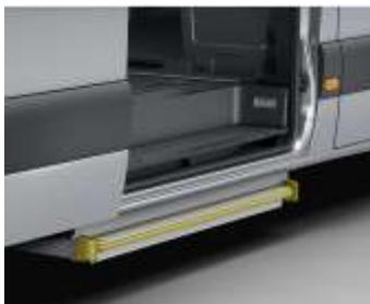
The electric step automatically extends when the sliding door opens, and retracts after the sliding door closes. This operation is possible without a use of the ignition key. The electric step is 47.24" (1200 mm) width and 11.42" (290 mm) depth. The maximum permissible capacity is 330 lbs. (150 kg). The aluminum step with a hot-dip galvanized cassette has a self-weight of 92 lbs. (42 kg).
