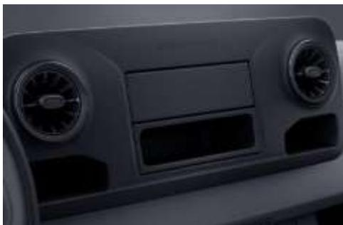
The radio fittings provide an AM/FM antenna, a 12 V power source and the interface for 2-way loudspeakers in the front. A single DIN slot is provided in the center of the cockpit for retrofitting a radio. The pre-installation for radio does not support CAN technology. Without CAN e.g. the control of the radio via the multi-function steering wheel and display of radio information in the instrument cluster are not supported.
