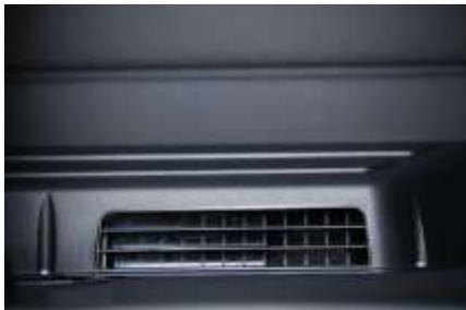
The hot-air duct to the rear passenger compartment is installed between driver and co-driver´s seats. The hot air duct supplies the rear passengers with warm air when the air distribution control is set to ventilate the foot well.
