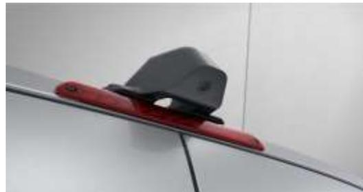
Trailer mode supports the driver when reversing to a trailer by zooming to the trailer hitch. To do so, special guide lines are shown in the display in addition to the pictures recorded by the reversing camera.
