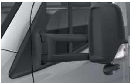
The exterior mirror is mounted on an extended mirror arm which improves rearward visibility, in case an extra-wide body is fitted. Code FS1 is for a vehicle width of 86 - 90" (2184 - 2286 mm)
