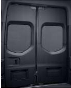
The matte black washable plastic paneling is available for the right-hand sliding door and for the hinged rear doors. This paneling completely covers all metal parts; therefore, improving a visual upgrade of the passenger compartment. In addition, it improves the sound and heat insulation.
