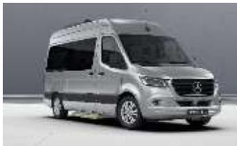
The rear windows, and all side windows in the rear section, are dark gray-tinted (approximately 90% tinting). The windshield and the windows in the driver's and co-driver's doors are green-tinted.
