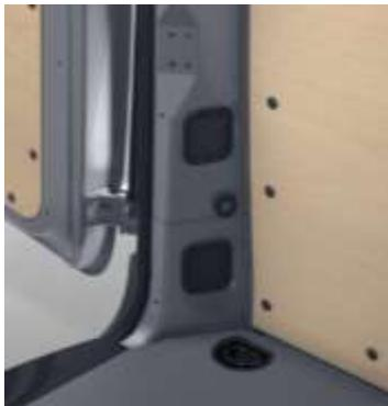
A 12-volt socket is located in the left-hand D-pillar trim of the passenger/cargo Van. The passenger Van also has a 12-volt socket in the right-hand D-pillar trim. Both sockets have a maximum power rating of 180 watts. Power can be drawn regardless of ignition key position. The sockets are supplied with power by the starter battery, except if code E21/E2M is specified, in which case it is supplied by the auxiliary battery.
