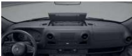
This equipment allows the customer to store items out of sight allowing for a tidy atmosphere. The center storage compartment on the instrument panel may be fitted with a hinged lid via code FJ1. Complementary to this code, FJ5 offers two hinged lids for storage compartments on the left and right side. The cup holders on the left and right outside are then omitted.
