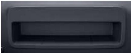
The code FJ7 includes a large storage compartment in the upper central area of the instrument panel and is only available when the air conditioning system code HH4/HH9 is omitted. The dimensions of this storage compartment are 18.11 x 3.94 x 4.72" (460 x 100 x 120 mm) (Width x Height x Depth).
