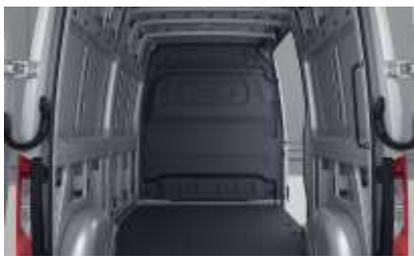
The full width sheet metal (steel) partition D50 located on the B-pillar is designed as one-piece for standard height roofs and two-pieces for high roof versions. These two options now have a 0.59" (15 mm) deeper contouring at backrest height. This allows for the front seats to be better adjusted to the driver and co-driver's comfort and provides a solid barrier for cargo, noise and dirt.
