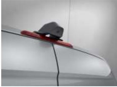
An additional LED brake light is fitted at the rear edge of the cargo van or passenger roof. The third brake light does not affect the height of the vehicle at the rear.
