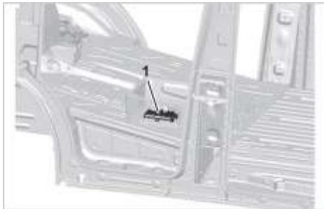
The main fuse box now contains four additional fuses (40/80/80/100 Amps) that are not utilized by the Sprinter and are dedicated fuses for electrical consumers on upfitted vehicles. Please look at the Sprinter operator's manual for more information on fuse locations.
