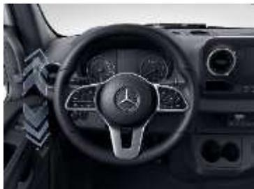
The steering wheel is manually adjustable for tilt and height. To provide a large adjustment range, the wheel can be tilted at a vertical angle between 28 and 32 degrees and adjustable axially by 2.36” (60 mm) and 1.96” (50 mm) in height. The adjustment is performed by a lever on the steering column.
