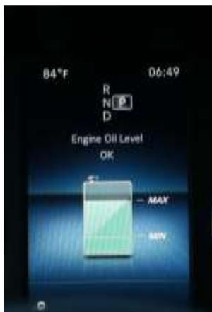
When parking the vehicle for a longer period of time, the last saved oil level is displayed at the start of the engine. The notification must be acknowledged by the driver. In addition, the oil fill level can be accessed via the service menu on the instrument cluster. It also scans a too low/high oil level in order to prevent engine damage.
