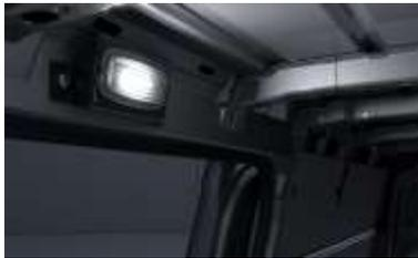
Two additional ceiling lights are fitted at the roof frame on the side wall. A door contact switch turns the lights on/off when the load compartment doors are opened/closed. The lights can also be switched on/off by the switch in the overhead control panel. In combination with code LC2, all standard ceiling lights in the load compartment come as LED.
