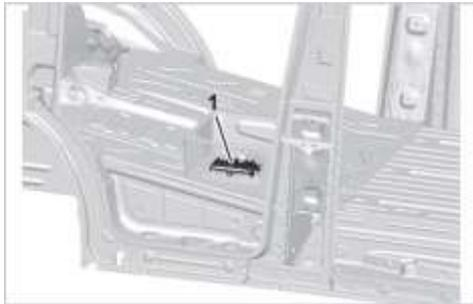
The main fuse box now contains 4 additional fuses (40/80/80/100 Amps) that are not utilized by the Sprinter and are dedicated fuses for electrical consumers on upfitted vehicles. Please look at the Sprinter operator's manual for more information on fuse locations.
