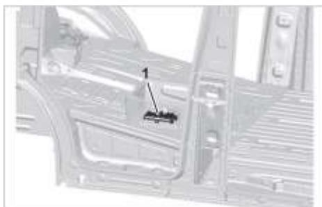
The main fuse box now contains four additional fuses (40/80/150/100 Amps) that are not utilized by the Sprinter and are dedicated fuses for electrical consumers on upfitted vehicles. Please look at the Sprinter operator's manual for more information on fuse locations.
