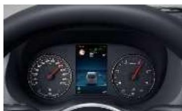
JK5 has two large chrome-lined analogue displays for vehicle speed in km/h or mph, engine rpm, fuel fill level, and temperature. A centrally placed high-resolution 5.5" color display allows the driver to easily view and browse the menu using the upper left touch-control panel on the multifunctional steering wheel.
