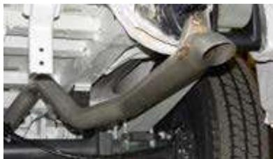
The vehicles come with a straight exhaust up to the rear as standard via code K60. The exhaust ends shortly before the rear of the vehicle and prevent unpleasant odors in areas of boarding and alighting.
