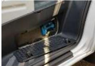
The hydraulic jack facilitates jacking up the vehicle to change a tire. It is located in a bracket in the entrance area on the passenger's side and is easy to remove.
