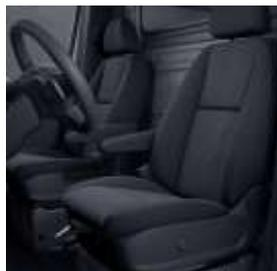
The lumbar support in the backrest of the driver's seat enables the seat to be adjusted to suit the driver's ergonomic comfort requirements. Both air bladders are adjusted pneumatically. The height of the bladders and the extent of the curvature can be controlled with a 4-way switch at the outside of the driver's seat. This optional feature is available for 3 seat variants. Seats fitted with lumbar support meet the criteria of the German AGR campaign for healthy spines.
