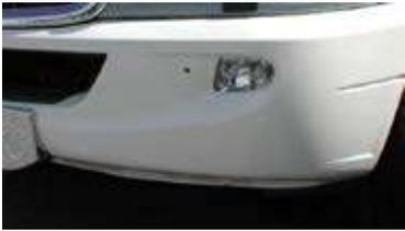
The entire bumper is painted pure white (MB 9678). This coating makes it possible to apply a topcoat in any desired color.
