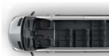
A three-seater comfort bench is fitted in the **third** row of the 14+1 passenger compartment and can be optionally selected. All three seats are fitted with a three-point seat belt and have additional seat bolter padding, allowing for enhanced seating comfort. Each row is individually reclinable as well as an individual recliner setting on each seat.
