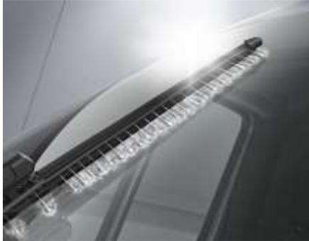
The adaptive wind-screen wiper system provides the driver with an ideal view - even during the cleaning process. The cleaning fluid is sprayed directly in front of the wiper blades through its small nozzles and is wiped away immediately. In result of the directed distribution, the amount of cleaning fluid needed can be reduced by up to 50 % while still obtaining ideal cleaning results.
