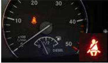
The seat belt warning for driver's seat, code J58, is now complemented by the seat belt reminder for passenger seat, code J55. The seat belt reminder for driver and co-driver increases the passive safety level. An optical signal in the instrument cluster reminds the driver or co-driver to buckle up when starting the vehicle. If this is ignored and the vehicle is in motion 15 mph (25 km/h) an acoustic signal sounds.
