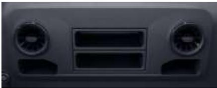
The code FJ6 includes two DIN storage compartments and two additional air vents in the upper central area of the instrument panel. Each air vent can be individually adjusted. This layout of the central area is standard for vehicles without pre-installation for radio or multimedia system. The dimensions of the storage compartments are 3.94 x 1.77 x 3.94" (100 x 45 x 100 mm) (Width x Height x Depth).
