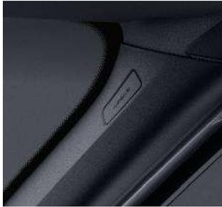
The window airbag units are installed along with the associated filling pipe at the inside of the respective roof frame behind the A-pillar paneling. The window airbags can protect the head area of the front passengers on the affected side in the event of a side impact. The code SJ3 deletes the co-driver's window airbag. In this case only the driver's window airbag is installed. This allows special-purpose vehicles with modified passenger section.
