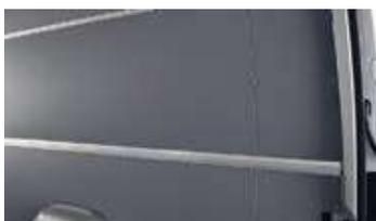
Bonded lashing rails are fitted along the side walls of the vehicle at hip height at approximately 28.5" (724 mm) and also the roof frame at approximately 64.4" (1636mm) with a distance between the two of approximately 38.9" (988 mm) below the roof frame. The holes in the lashing rails are spaced at approximately 1" (25 mm) intervals. Straps are not included in the specification, but are available as accessories. Load rating is 1,500 N (335 ft-lbs.).
