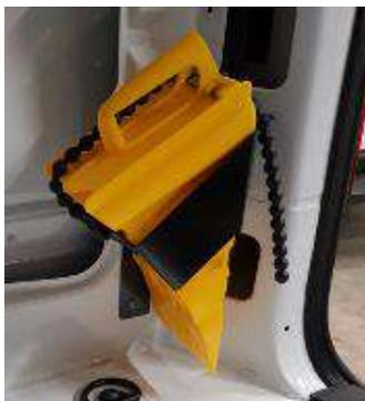
Cargo and passenger van models have a chock holder mounted on the D-pillar at the rear right of the cab. Cab chassis models have a chock holder mounted on the left at the frame end.
