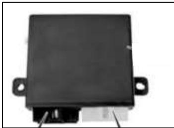
The parameterizable special module (PSM) gives upfitters access to individual types of CAN bus data. The PSM is able to read messages of the various bus data and then, for example, translate them into switching signals at the outputs provided or PWM signals or forward those to a specific body manufacturer upfitter CAN. The installed electronics then have access to the necessary signals.
