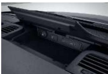
The charging package expands the charging facilities in the cockpit to two 5 V USB-C ports and one 12 V power socket. One of the USB ports as well as the 12 V socket are located in the center storage recess of the instrument panel. Another USB port is located in the lower part of the center console. This allows for charging of electric devices such as mobile phone within the driver's and co-driver's reach.
