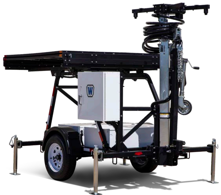
Storage position with drawbar up, 1500-watt model
