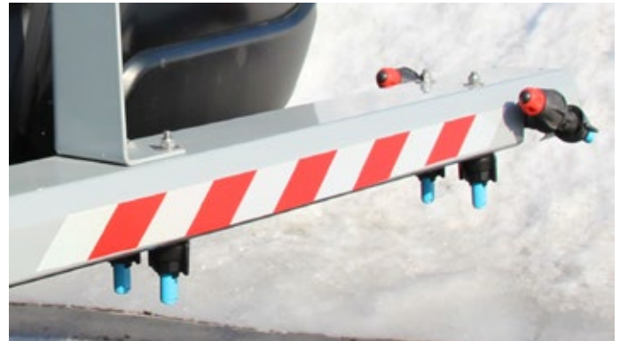
Double spray nozzles for de-icing even at higher speeds.
