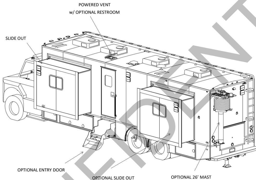
**Note that the above is picture is a representation of a Nomad IC32 Mobile Command Vehicle. If there is a discrepancy between the drawings and this SOW, the SOW will take precedence.**
