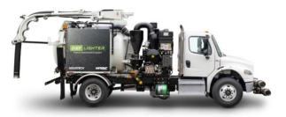
Boom mounted internal air Vac valve Boom clean out port
