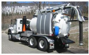
Boom mounted internal air Vac valve Boom clean out port
