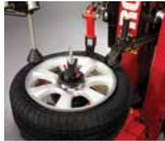
**EASY TIRE MOUNTING** with plastic tool, dual rollers and power-assisted top bead press arm.
