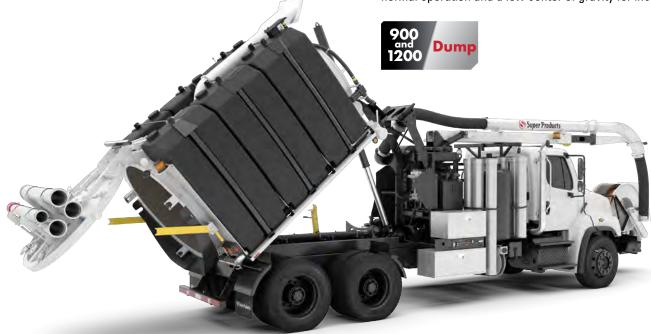
**Eject Unloading:** The eject unloading system is the industry's safest and most efficient removal of debris. The body raises to an 8.5° angle and the ejector plate quickly pushes out debris. This allows operators to have **the only controlled way to dump into a 48-inch container** without the need of additional containment products.
