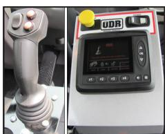
Joystick, mounted in the armrest of the truck for easy access, controls the boom direction, speed, engine throttle and box container dump. a
