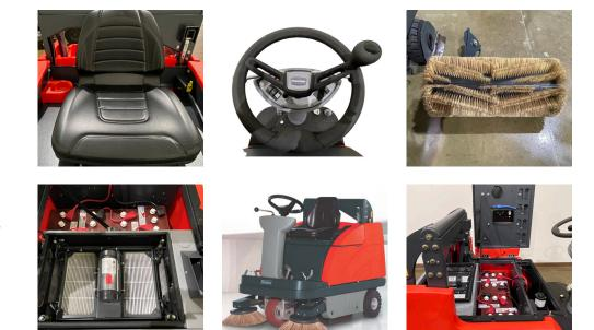
Increase sweeping performance with the Apex 47- Front wheel steering and the upfront operators station ensures excellent visibility for cleaning.
