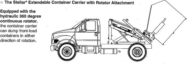
The center of gravity of the ECCR unit is located approximately 9.25" in front of the rear axle. In the stored position, the center of gravity of the container is located approximately 45" behind rear axle.
