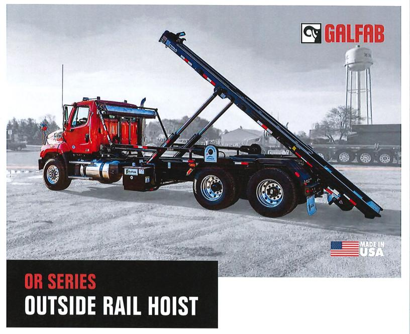
The Outside Rail roll-off hoist is the most commonly used hoist in the industry today. GALFAB offers this hoist with an 8" mainframe and 2" subframe or the very popular 10" sub frameless hoist.
