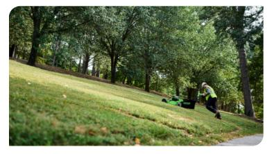
ETS DRIVE SYSTEM: DUAL INDEPENDENTLY CONTROLLED HUB MOTORS AUTOMATICALLY ADJUST THE POWER TO COMPENSATE FOR SLOPED CONDITIONS FOR EFFORTLESS CONTROL.
