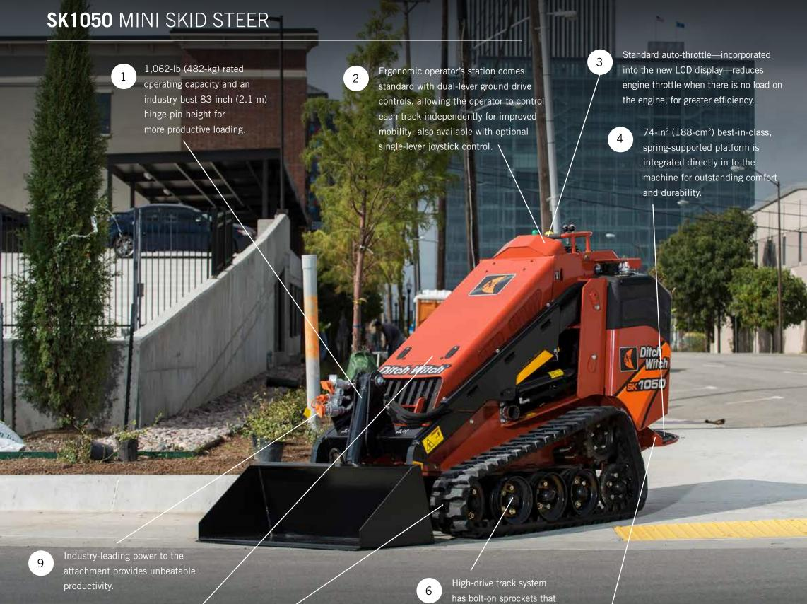
Ideally suited for a variety of demanding jobsites, the Ditch Witch® SK1050 mini skid steer improves versatility and productivity by directing more hydraulic power to the attachment. The durable, construction-grade design eases operator maintenance for improved ROI, and outperforms all other working machines in its class. Designed specifically for the hardworking operator in mind, the best-in-class, spring-loaded operator platform improves comfort for long hours on the job.
