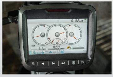
An easy-to-read 7-inch LCD display panel displays critical machine data, errors, warnings, and the rearview and sideview camera display. It also has an automatic night view function for optimal visibility in low light conditions.
