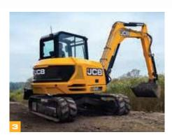
The heavy duty boom cylinder guard provides excellent protection with optional dipper and crowd cylinder guards available for more arduous applications.
