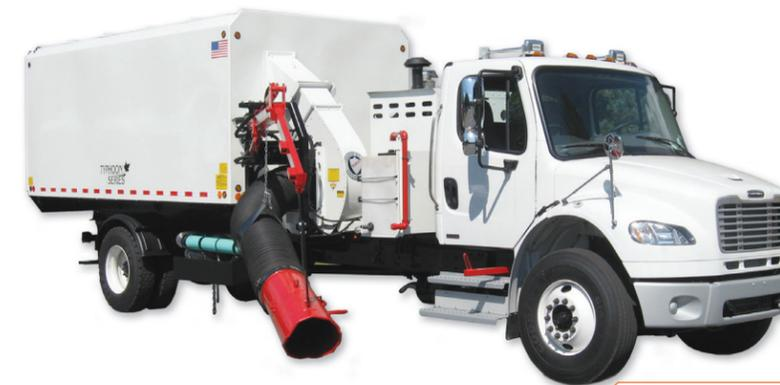
our other TARCO® brands. Standard features include: rugged body construction for durability and extended life, heavy duty 6 blade suction impeller, curb side pickup, built-in operator and equipment safety mechanisms, grip notched power belt drive to protect engine and PTO, and John Deere diesel engines, to ensure premium performance and reliable local service.
