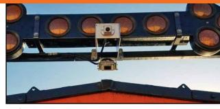
360° rear camera and 10" monitor with mobile digital recorder. Wi-Fi and 4G Compatible.
