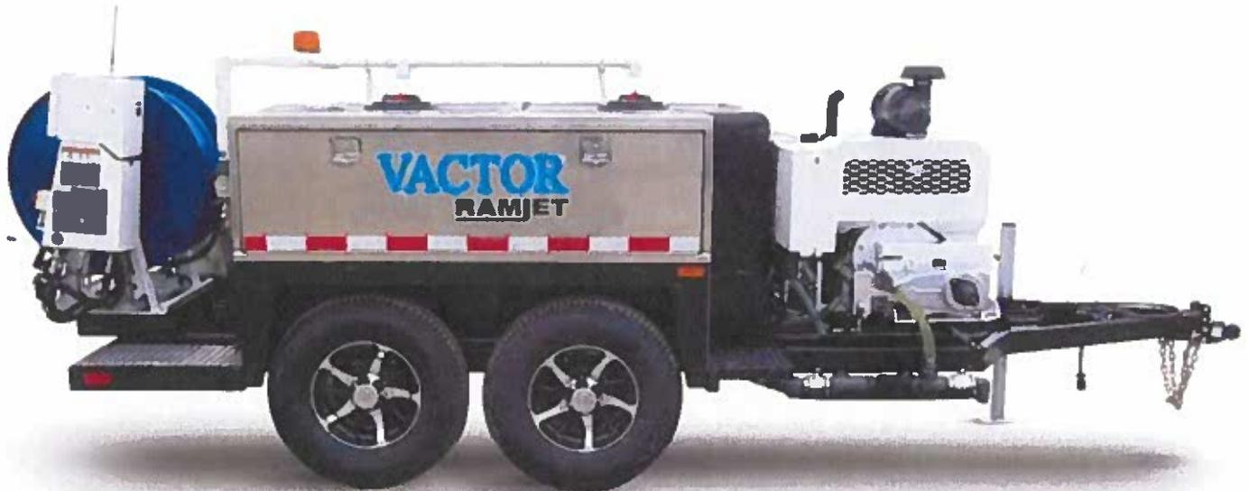
The Ramjet trailer & skid-mounted jetters are the perfect machines for fast, safe response to sewer blockages as well as regular preventative line maintenance. Our line of reliable, high-pressure water jetters are specially designed for cleaning municipal sewer, drain and pipe lines as well as culverts at low water volume. These units are ideal for cost effective maintenance and emergency response in tight, confined environments.
