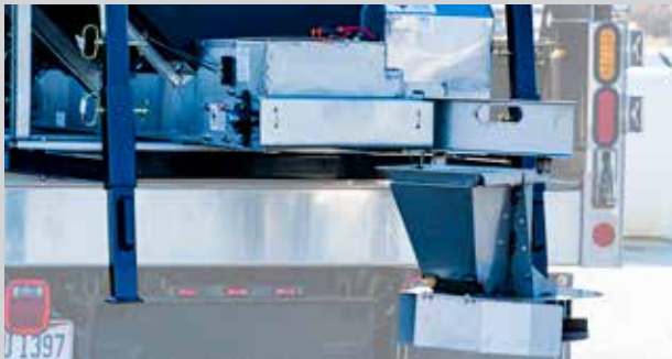
Swing away chute for easy cleaning, storage, and bulk unloading
