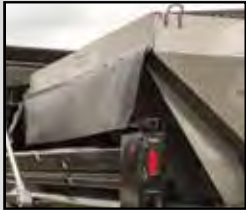
Optional Rubber Side Deflectors Part No. 1492144
