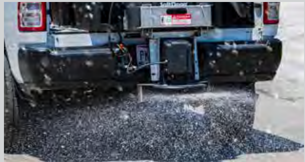
Two 12V direct drive gear motors (3/4 HP for auger or chain and 1/2 HP for spinner)
