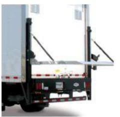
allows platform to travel above truck bed-height for dock loading
