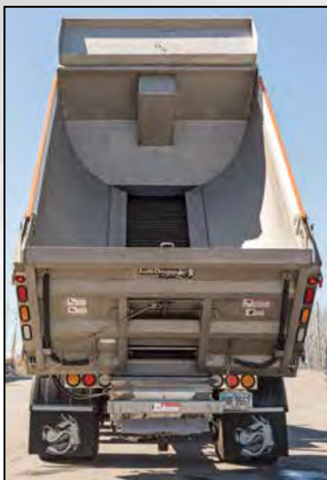
Unique, roll-formed sides and cross member-less design
