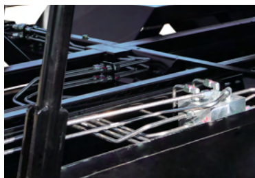
*Patent pending hydraulic fluid line for tarper system.
