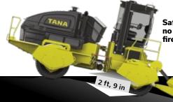
Safe design without belly pans: no debris accumulation to cause any fire hazards.
