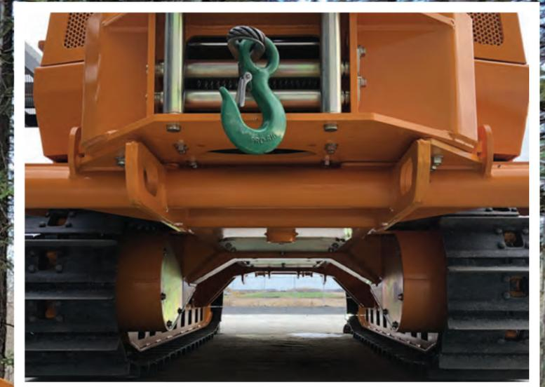
CLEAR THROUGH BOTTOM WITH HIGH GROUND CLEARANCE AND NO CROSS BEAM
