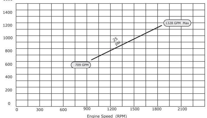
The above curve is based on pumping clear water at 62 degrees with no lift required and no restrictions in the discharge.
