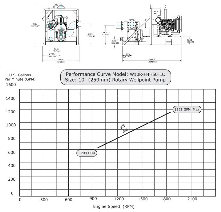
The above curve is based on pumping clear water at 62 degrees with no lift required and no restrictions in the discharge.
