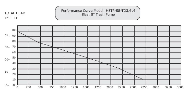
U.S. Gallons Per Minute (GPM) @ 2000 PSI
