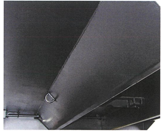
Pictured is the crossmemberless understructure of the 433USS using 3/16" X 100K formed 10" trapezoidal longbeams
