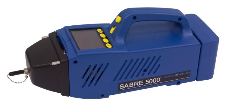
The **SABRE 5000** is the smallest, lightest tri-mode handheld system available for detecting trace amounts of explosives, chemical warfare agents, toxic industrial chemicals or narcotics. With its ability to detect a wide range of threats, it is a cost effective instrument for security professionals and military agencies that require portability and flexibility to perform their duties.
