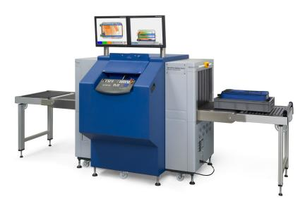
The *HI-SCAN 6040-2is* is an advanced dual-view X-ray inspection system for automatic explosive detection at check-points where bags and personal belongings are screened to protect society. It utilizes proven Heimann X-ray technology to automatically detect explosive materials and generate reliable, high quality dual-view images.
