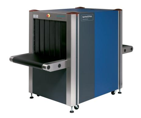
The *HI-SCAN 7555i* is a compact x-ray inspection system with a tunnel opening of 755 mm (30") wide by 555 mm (22") high. This tunnel size is ideally suited to screening checked luggage and packages as well as briefcases, handbags and other small items.
