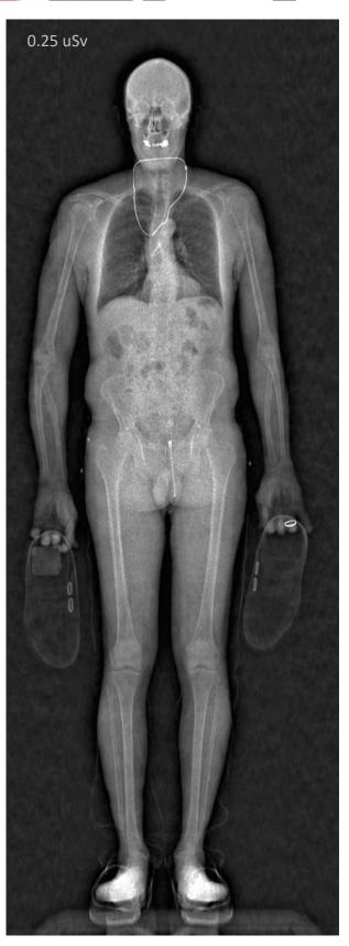
A typical image from Intercept on the lowest setting, 0.25  $\mu$ Sv. Intercept can operate at up to 200  $\mu$ Rem for even better image quality. Items: teeth fillings, neck chain, object in shoe heal, ring, and zipper.
