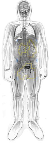
This intelligent software analyzes the X-ray images received on CONPASS Full-body scanner and highlights torso area in which narcotics may be hidden by a suspected trafficker. This sophisticated software accurately identifies and alerts the operator to the presence of suspected narcotics. Currently deployed at correctional facilities, airports, and border crossings, it has proven to be a a valuable tool to assist law enforcement personnel in drug interdiction efforts.
