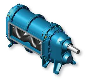
**Vibration:** Pumps and motors operate at any point within their operating range without undue noise and vibration **Top and Bottom Housing Segments:** ASTM A48 Class 30 gray cast iron coated with ceramic epoxy for wear resistance; options include Ryton<sup>®</sup> and Tungsten Carbide. Segments adjustable based on wear.
