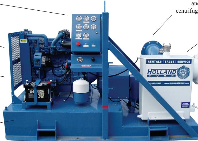
**Steady Discharge Flow** ensures continuous output and discharge against head versus competing centrifugal pumps that surge and have lower output
