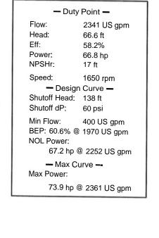
Data shown in table and curve is based on approximate pump performance at sea level with 60° F water. Larger diameter pipe may be required for maximum flows.
