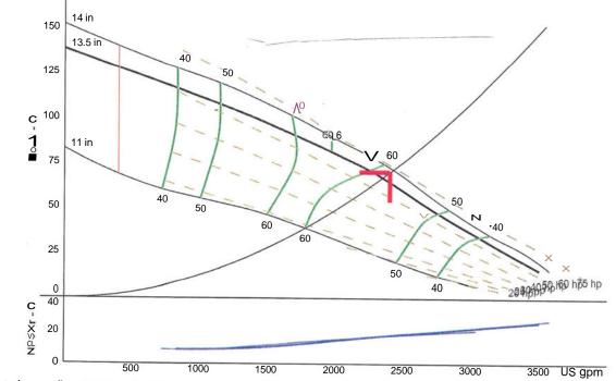
Min flow line represents the absolute lowest flow pump can operate. Consult with factory if operating below
