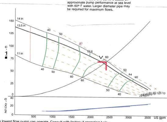
Min flow line represents the absolute lowest flow pump can operate. Consult with factory if operating below
