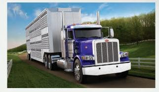
The Model 389 features conventional styling, plus a selection of components and options for efficiency and performance. Peterbilt's lightweight and durable hood is the industry's only all-aluminum hood with a distinctive punched oval grille and one-piece aluminum crown.
