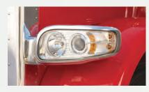
**VISIBILITY** Halogen projectors, aluminum headlamps and long-life LED directional signals are protected with an impact-resistant lens and contribute to overall exceptional visibility.
