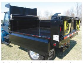
Optional drop sides in the down position. The side easily unlatches with a single handle and folds down lower than the body floor. Body shown with additional options.
