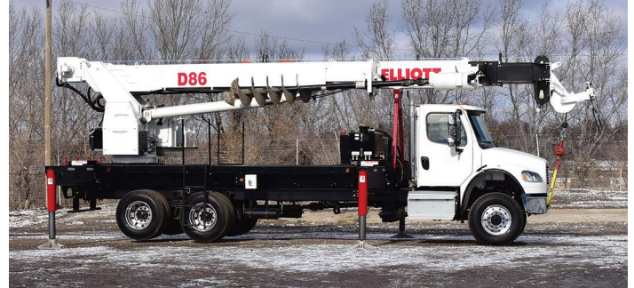
Chassis data is minimum general requirements-not for engineering. Actual dimensions and truck data will depend on truck selection and axle configuration. *Minimum chassis weight is required to meet 85% stability requirements.
