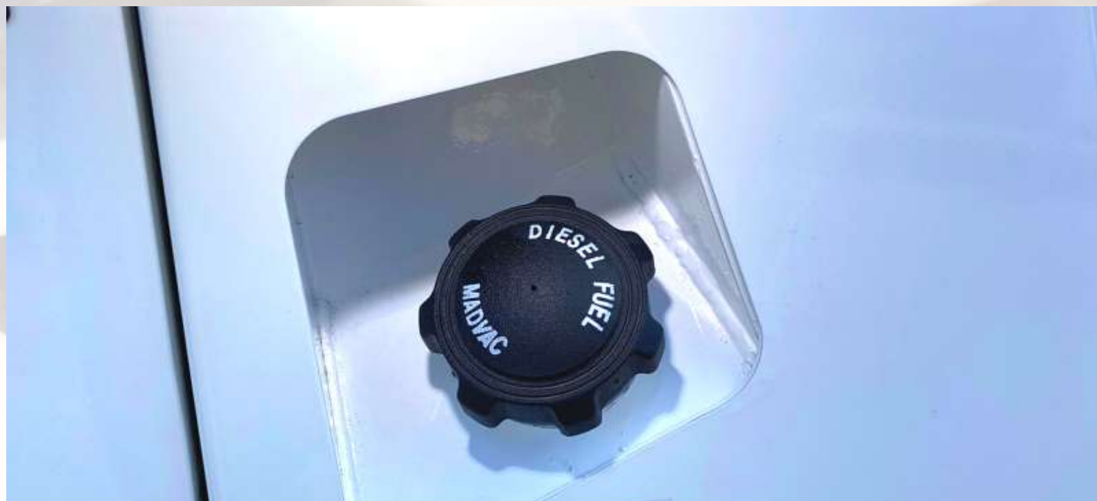
Diesel fuel tank filler
