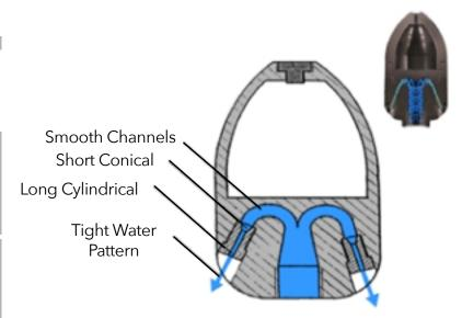
It is easy to see that as we follow the path of water through a KEG Tier Three Nozzle, our high-performance design leaves little room for excessive turbulence and power losses.
