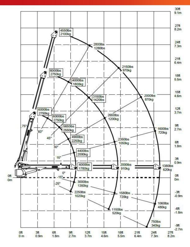
Weights of load-handling devices are part of the load lifted and must be deducted from the capacity.
