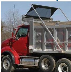
11525 – Steel 4-Spring External Mount System Covers up to 24' or less 11567 – Steel 5-Spring External Mount System Covers up to 26'
