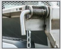
3/4" Diameter stainless steel tailgate hitch pins
