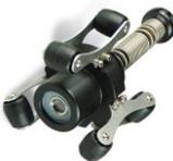
Use Mini-Cam Roller Skids to increase the effectiveness and lifespan of your pipeline inspection system. Simply fit the skid and the three pivoting arms with specially shaped nylon wheels keeping the camera head centered in the pipeline at all times.
