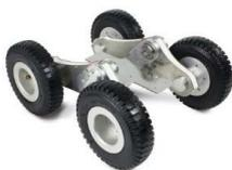
For use with the CRP140 or CPL150 crawlers. Quickly attach the crawler to extend its capability from 600mm up to 1,050mm. Features a unique gear selector to choose between high speed lower torque or lower speed higher torque. Comes supplied with 4 x 220mm & 4 x 250mm balloon wheels.
