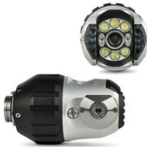
High resolution camera module, extremely powerful LED lighting, Adjustable focus, pressurised, endless rotation, integral distance sensor and visible lasers to enable accurate pipe diameter, defect and object measurement. +/- 135° pan, pressure rated to 1 bar. 120mm x 73mm OD
