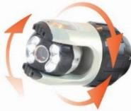
High resolution camera module, extremely powerful LED lighting, Adjustable focus, pressurised, endless rotation, +/- 135° pan, pressure rated to 1 bar. 120mm x 73mm OD
