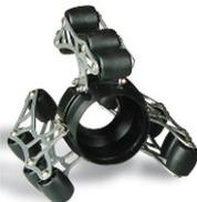
Use Mini-Cam Roller Skids to increase the effectiveness and lifespan of your pipeline inspection system. Simply fit the skid and the three pivoting arms with specially shaped nylon wheels keeping the camera head centered in the pipeline at all times.
