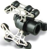
Use Mini-Cam Roller Skids to increase the effectiveness and lifespan of your pipeline inspection system. Simply fit the skid and the three pivoting arms with specially shaped nylon wheels keeping the camera head centered in the pipeline at all times.
