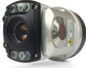
High resolution Zoom camera module with 10x optical, 12x digital zoom. Powerful LED Lighting, auto-focus, built in lasers for measurement, pressurised, endless rotation, +/-135° pan, pressure rated to 1 bar. 140mm x 80mm OD
