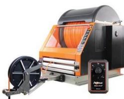
Fully automatic cable reel that holds 500m of cable, self-layering to keep the cable neat and tidy. Removable drip tray. Fully synchronised with the crawler for hassle free pay and retrieval. Comes supplied with van mounted guide pulley and Joystick Bluetooth remote control (RJP01).
