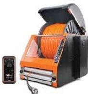
Fully automatic cable reel that holds 350m of cable, self-layering to keep the cable neat and tidy. Removable drip tray. Fully synchronised with the crawler for hassle free pay out and retrieval. Comes supplied with Joystick Bluetooth remote control (RJP01). Please note: Van mount guide pulley (VGP350) must be ordered separately if needed.
