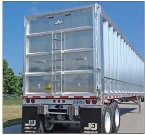
Standard bumper with extra wide blocks protects the trailer from damage due to many years of tipping.
