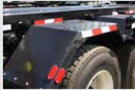
Steel, aluminum or poly fenders
