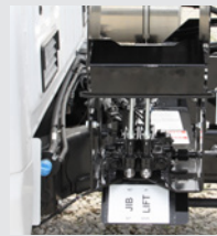
Secondary outside manual control valve with protective cover
