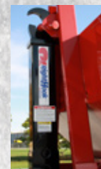
T-1 steel fixed hook height @ 54"
