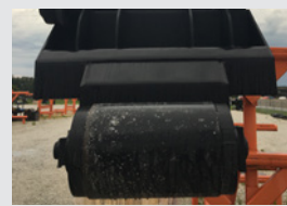
Rear hydraulic activated stabilizer with 10" ground roller
