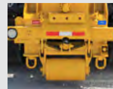
Rear hydraulic stabilizer with 10" ground roller
