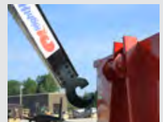
T1 steel fabricated fixed hook height at 61 ¾"
