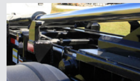
Outside frame rail stationary rear container hold downs
