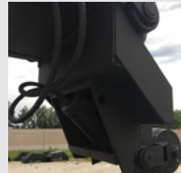
Rear hydraulic activated stabilizer with 10" ground roller
