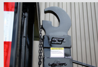
Pull (2) pins to slide in/out dual hook height adjustment
