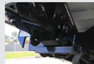
Twin locking mechanism for dual pivot activation
