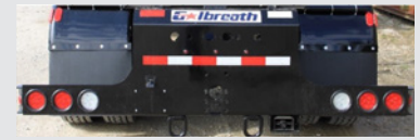
One piece rear apron / bumper with LED lighting and pintle / reese hitch adaptable
