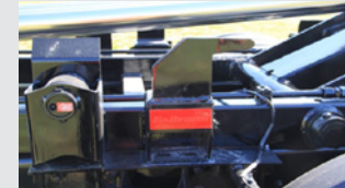
Welded & bolted on roller stools with 4" OD rollers & bronze bushings
