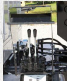
Secondary outside manual control valve
