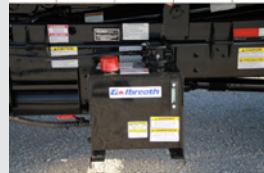
Steel tank with dual sight/temp gauge and air breather
