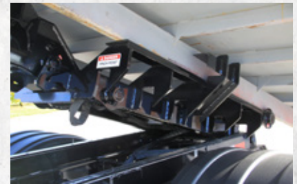
Rear container transition supports w/ pass through rear hold downs
