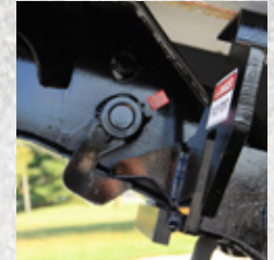
T-1 steel fixed hook height @ 54"
