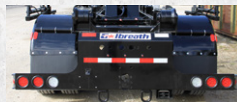
Rear apron & bumper assembly complete w/ LED lighting & pintle/reese adaptable
