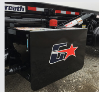
50-gallon steel hydraulic tank side mounted with dual sight / temp gauge
