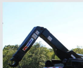
T1 steel hook, adjustable bolt on from 54" to 61 ¾"
