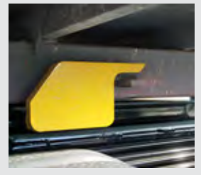
Outside frame rail stationary rear container hold downs
