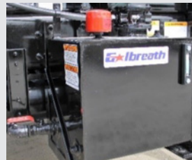
Steel tank with dual sight/temp gauge and internal return filtration
